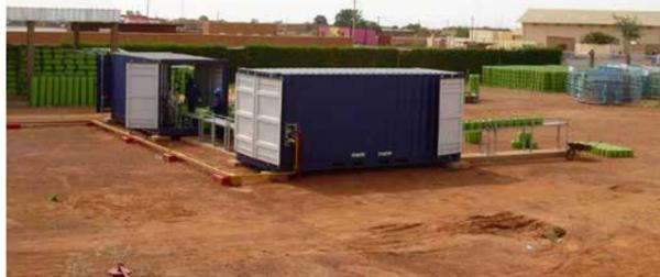
Container with check equipment and roller conveyor for loading/unloading
