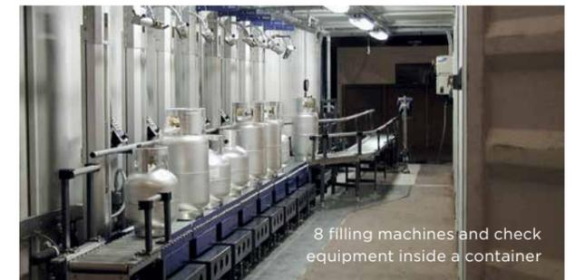
8 filling machines and check equipment inside a container
