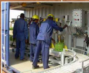
A fully equipped filling container with 1-8 filling machines
